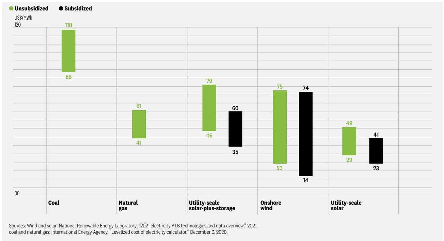
**FIG 2:** New-build renewable energy vs. marginal cost of existing conventional generation
