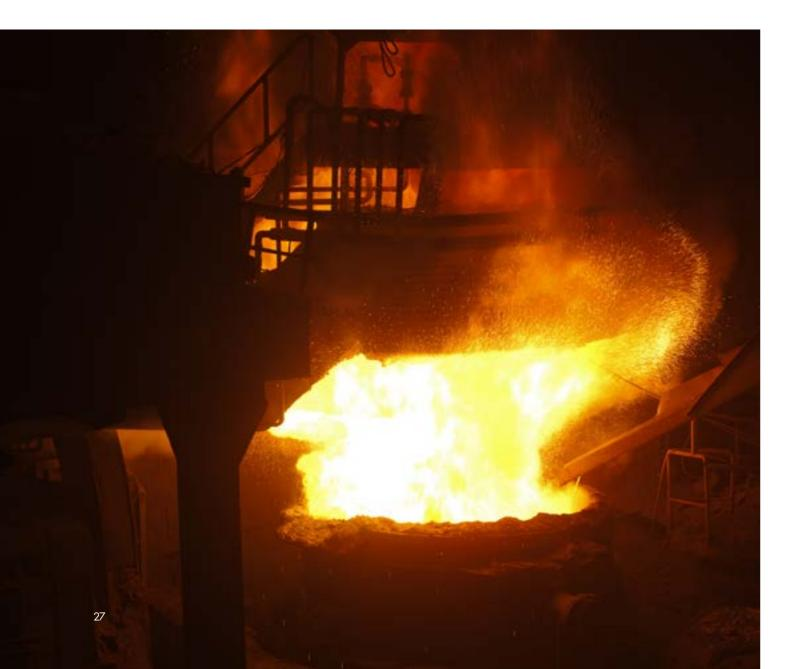
DRI-EAF production plants require higher-quality iron ore than BF-BOF plants, because insufficiently dense iron ore can create acidic slag which can corrode the electric arc furnace and, in the longer term, lead to decreasing vields.
