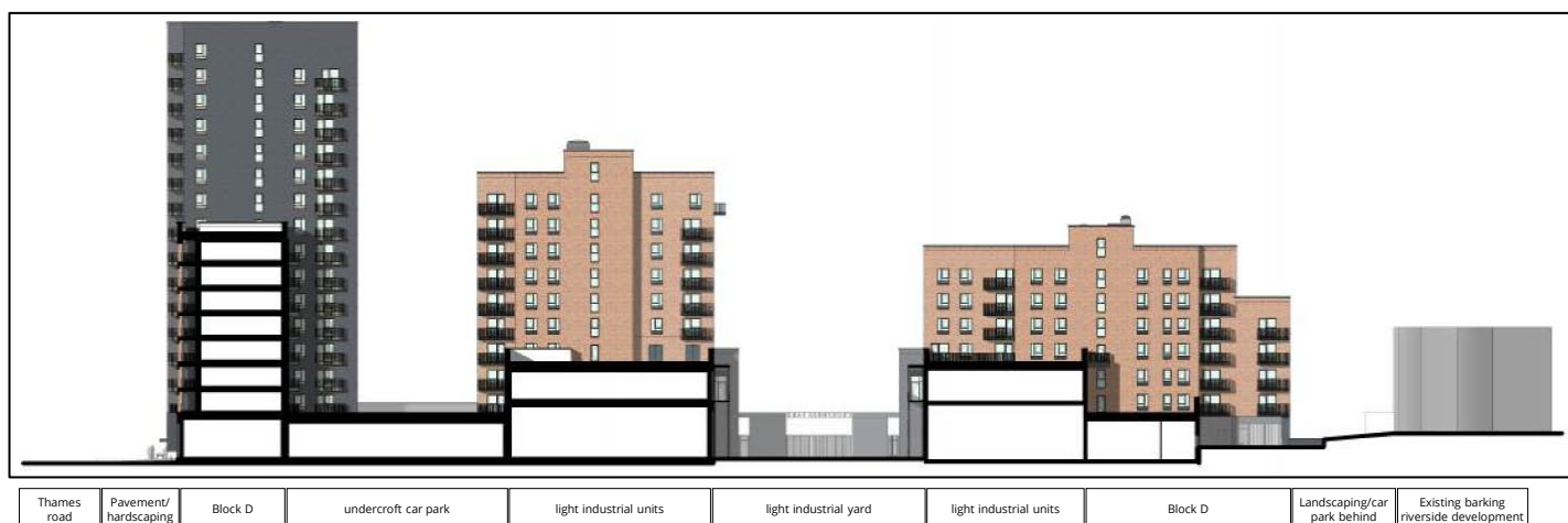
Figure 5: Elevation/section of the 12 Thames Road development, illustrating the location and height of the ground floor industrial element relative to the homes. Balconies for the homes are orientated facing away from the industrial yard space to minimise noise impacts. (Source: BPTW)
