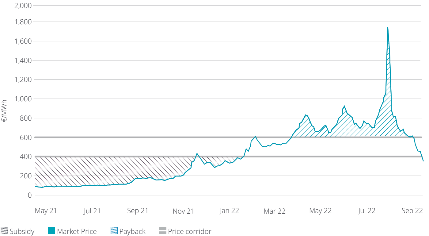
Fig. 21 – Illustration of Contract for Difference (CfD)
