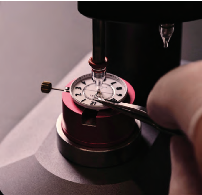
Manufacturing operation on watch hands. Photo courtesy of G&F Châtelain.
