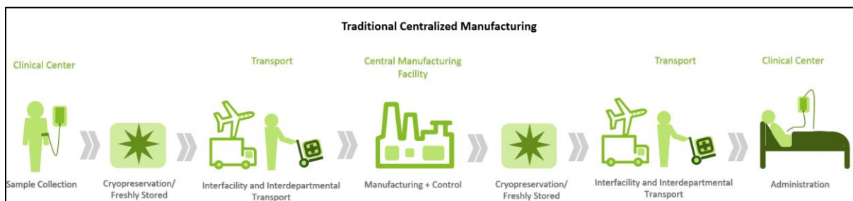
Figure 2a. Centralized Manufacturing. Centralized manufacturing of Cell and Gene Therapies starts with sample collection from the patient in the hospital/clinical center. The cryopreserved or fresh material travels via interfacility and interdepartmental transport to the central manufacturing facility. Final products are then again cryopreserved or freshly stored and transported back to the clinical center where they will be administered to the patient.
