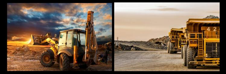
Diesel-powered equipment is used in open cast mining for drilling, loading and hauling material. The majority is used by haul trucks to move ore and mine waste. Mine pit depths vary from tens of metres to hundreds of metres with haul trucks loading hundreds of tonnes per round-trip. As a result, fuel and lubricants can account for about 40% of the operational spend for a typical mine.
