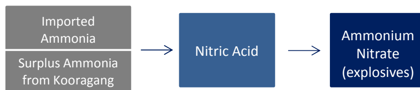
Figure 5.2: Production of ammonium nitrate at Yarwun, Queensland
