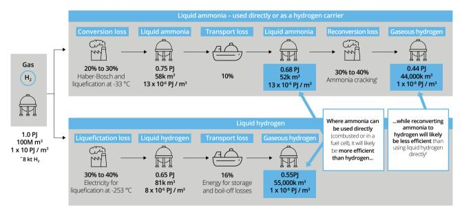
Notes: I) Ammonia cracking is energy intensive, requiring temperatures of >500 °C; II) Hydrogen use after reconversion also has downsides, as PEM fuel cells (e.g., in trucks) are vulnerable to trace amounts of NH3, requiring additional separation and purification
