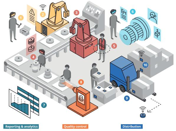
7 All devices are connected to a data management system, which digitally documents each step of the process. Advanced analytics predict demand patterns to optimise production. 8 Machines use sensors, computer vision, and photogrammetry to evaluate products against standards.
