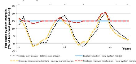
Figure 2: Evolution of the expected system margin for three market designs for one scenario of load growth (from Hary et al.) $^{9}$
