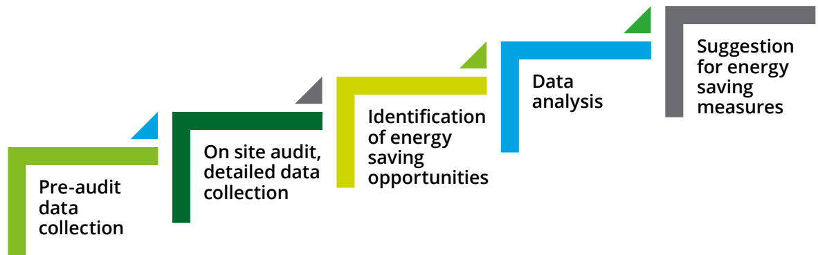
Figure 22: Process of a typical energy audit
