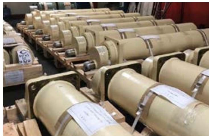
Initial Inspection of TBM Parts (16 Shield Jacks, 12 Articulation Jacks, 1 Main Bearing, 1 Cutter Reduction Gear and Motors)
