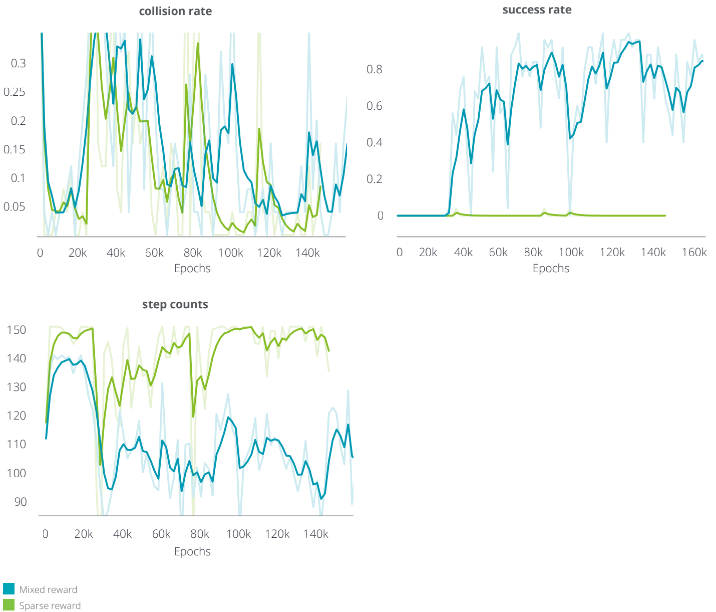
Fig. 3 – Performance criteria of a behavior planner over the reinforcement learning process for two different reward configurations. Learning using a mixed reward specification outperforms the sparse reward setting in terms of the share of successful scenario completions (success rate) and the time to complete the maneuver (step count). With mixed reward terms, however, the collision rate rises slightly. Adding additional continuous reward terms obscures the relationship between the specified collision reward and the resulting collision rate. As a result, it remains challenging to strike the right balance between behavioral specifications given by the ODD in the design of the reward system in our efforts to develop trustworthy behavior using reinforcement learning.
