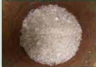
All of our seconds and reject plastic parts are reground in the granulator, then mixed with black masterbatch and injection moulded to produce small parts like tyres on toy trucks and bigger items such as high impact corners on outdoor toys.
