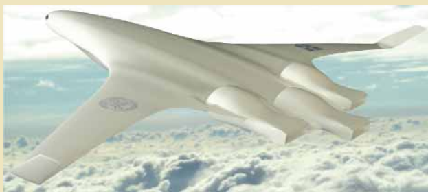
Figure 3: Impression of the “Integrated Wing” (courtesy of Silent Aircraft Initiative, Cambridge-MIT Institute, www.silentaircraft.org ).
